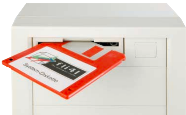
File4i packs a complete Linux router onto just one floppy disk
