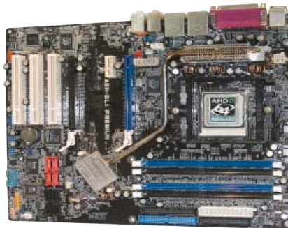
Asus is one of many vendors to offer fanless motherboards such as this A8N-SLI
