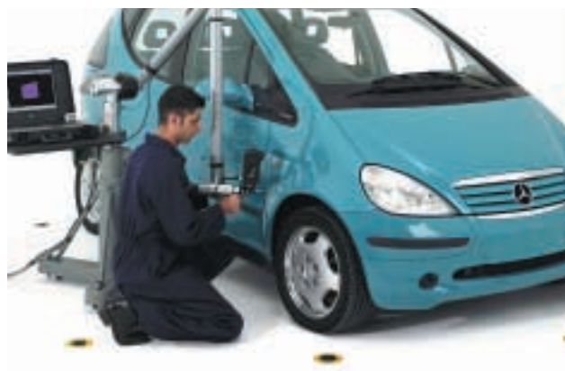
3D scanner in action mapping a Merc A Class
