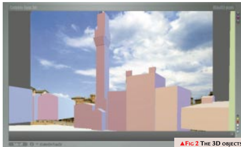
▲FIG 2 THE 3D OBJECTS CREATED USING THE PHOTOGRAPH, ALIGNED TO THE MAIN BUILDINGS IN THE SCENE
