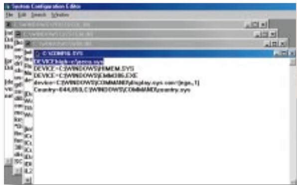
FIG 1 SYSEDIT IS A GREAT TOOL FOR EDITING ALL YOUR STARTUP FILES IN ONE HIT. HERE, THE CONFIG.SYS FILE IS LOADING THE DEVICE DRIVERS 'LOW' INTO CONVENTIONAL MEMORY. CHANGING 'DEVICE=' TO 'DEVICEHIGH=' LOADS THEM INTO UPPER MEMORY
