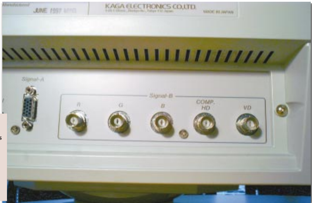
► Fig 2 THE SILVER COLOURED BNC INPUTS TO TAXAN'S ERGOVISION 750 TCO95 MONITOR CAN BE FOUND RIGHT NEXT TO THE 15-PIN D-SUB INPUT
