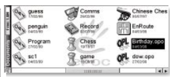
◀ FIG 5 ON THE PSION 5, YOU SHOULD FIND ICONS FOR THE 'COMPILED' VERSION OF YOUR PROGRAM WHICH, IF CLICKED, WILL RUN YOUR PROGRAM
