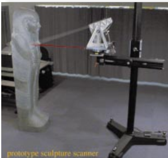
◀ FIG 3 THE PROTOTYPE OF THE 'RANGE' SCANNER BEING USED IN THE DIGITAL MICHELANGELO PROJECT, HERE BEING TESTED WITH AN EGYPTIAN SARCOPHAGUS
