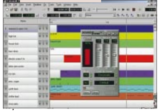
▼ FIG 4 SOUND 2 MIDI TAKES AN ANALOGUE SIGNAL FROM YOUR SOUND CARD'S EXTERNAL INPUT AND CONVERTS IT TO MIDI
