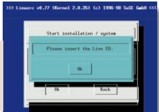
FIG 2 THE S.U.S.E 5.3 FIVE-CD PACKAGE INCLUDES A 'LIVE FILE SYSTEM' CD WHICH MINIMISES YOUR HARD DISK REQUIREMENT BY PROVIDING MOST OF THE ESSENTIALS READY-TO-RUN FROM YOUR CD DRIVE
