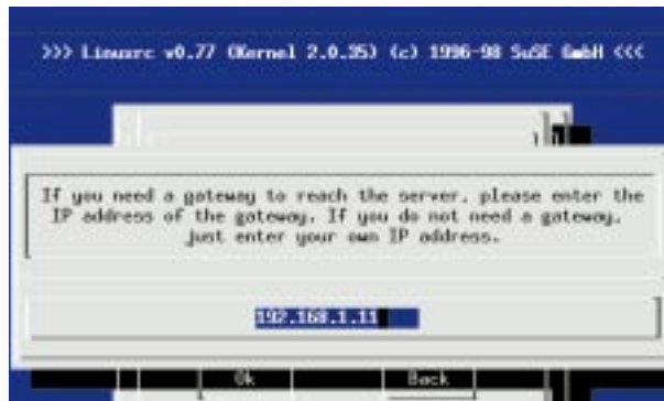
▲ FIG 3 IF YOU'RE USING A ROUTER, THIS IS WHERE YOU TELL S.U.S.E 5.3 ITS IP ADDRESS. IF YOU DON'T HAVE ONE, ENTER THE ADDRESS OF THE MACHINE ON WHICH YOU ARE INSTALLING
