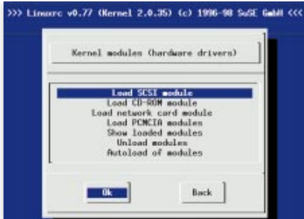
FIG 1 THE INITIAL PART OF THE S.U.S.E INSTALLATION RUNS A ROUTINE CALLED LINUXRC WHICH OFFERS A NUMBER OF CHARACTER-BASED SCREENS SUCH AS THIS, WHICH SETS UP FEATURES LIKE SCSI ADAPTERS AND NETWORK CARDS
