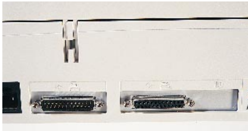
Parallel port scanners usually feature a "pass-through" connector for daisy-chaining a printer
