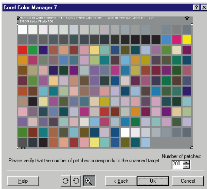
Fig 6 As with the scanner target, you need to tell the wizard where the corners of the printer target are so that it can match the swatches with the reference data and create the profile. The more patches you print, the more accurate will be the profile
