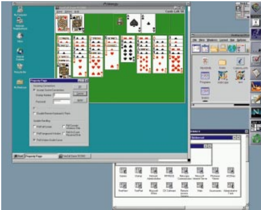
Fig 2 This is VNC, displaying the Primergy Windows NT screen on my IBM PC315, which is running Caldera OpenLinux. The display is a little more sluggish than a normal X window, but works well. The "Property Page" window can be used to control various features of the VNC server to optimise the display. The lower window behind is NTrigue, showing the earlier version of the Windows NT GUI
