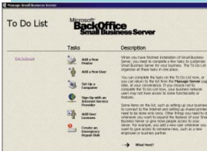
Fig 4 Microsoft Small Business To-Do List leads to web-based configuration dialogs for setting up and administering the server
