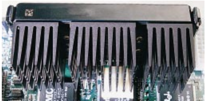
The traditional Pentium II with its familiar Slot 1, and toast-rack heat sink
