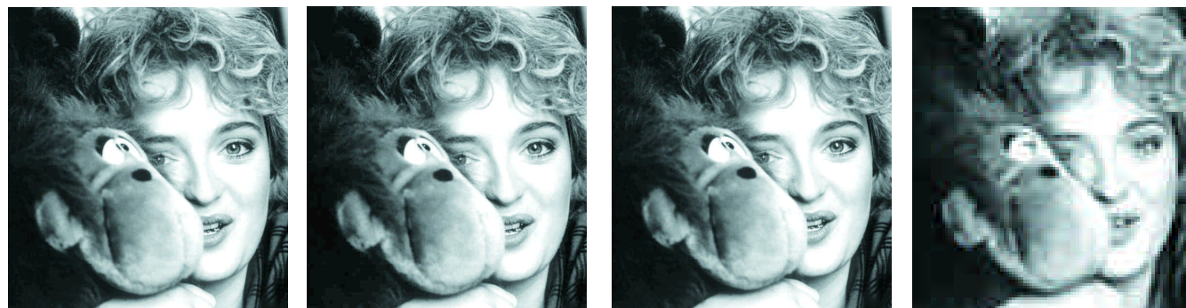
We started with a 300dpi greyscale image of 686Kb. Left to right: Saved firstly as a TIFF with LZW compression measuring 450Kb; secondly, saved as a JPEG with high compression measuring 47Kb; thirdly, saved as a GIF measuring 592Kb; and finally, an LZW compressed TIFF again, but this time reduced to 50dpi to measure 20.8Kb. Greyscale images are in 8-bit anyway, hence there is no loss in quality when saved as a GIF
