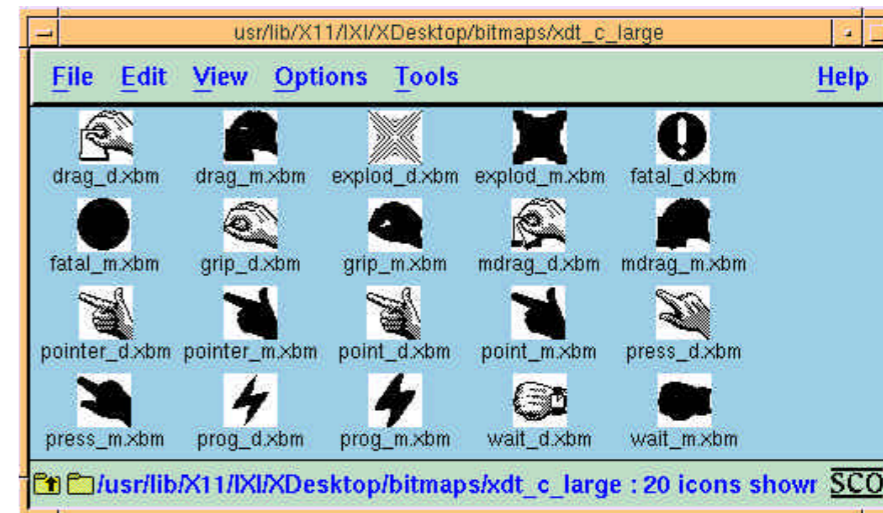
Fig 2 SCO: The pointing finger icon, which is the mouse cursor, pincers its finger and thumb to pick up objects, and rotates its wristwatch into view while waiting for a job to finish. Here are the icons that SCO's X.Desktop uses to do this
