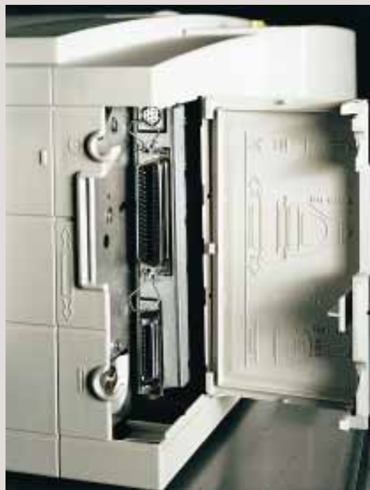
The rear of a typical printer. At the top is an Apple LocalTalk port for Macintosh computers, in the middle a standard PC parallel port. At the bottom is Compaq's new proposed standard for parallel ports
