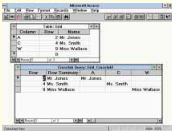
Fig 2 (top) Using a third table to create a many-to-many join between two others (see page 306)
